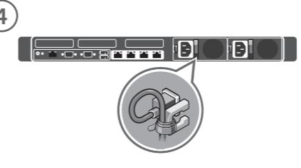
Loop and secure the power cable using the retention clip.
