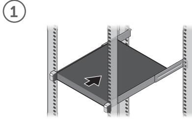
Install the system into a rack.
